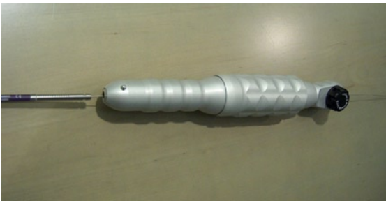
Before fixing the traction cable ensure that the handle is in neutral position. If needed , push the "release button" and adjust the handle.
