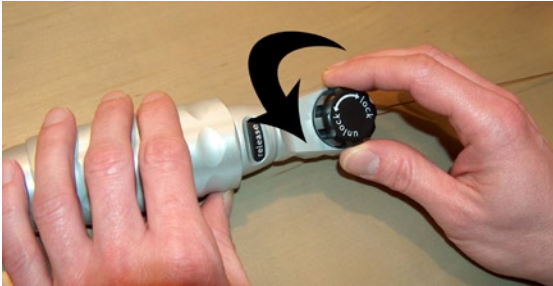
Open the black fixation device anti-clockwise and slide the handle over the traction cable .
